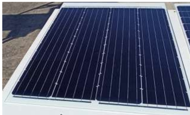
Figure 18 Shingled prototype assembled
