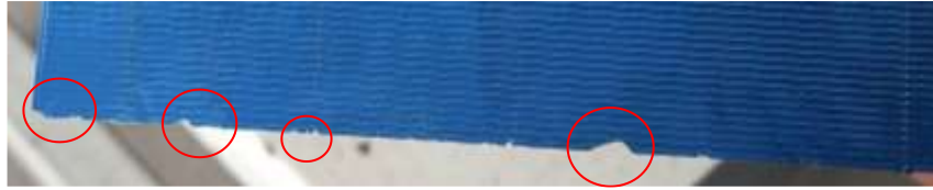
Figure 29 Polycrystalline cell damaged by the laser cutting process
